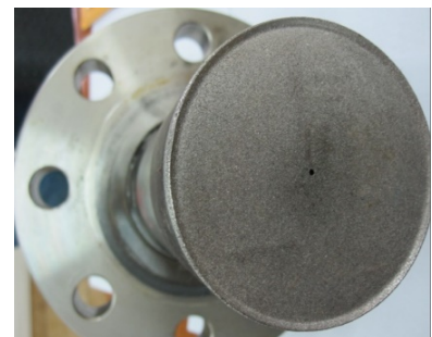
Figure 1: Hastelloy C276 diaphragm disappeared within one-year operation
