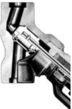
Disk Nut Construction - All Univalves and Post 1991 Bolted Bonnet Valves
