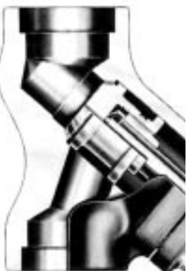
Disk Nut Construction - Bolted Bonnet Valves - Pre 1991
