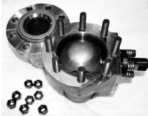
5) Remove body nuts and separate body and end cap.
