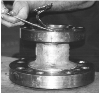
7) Remove body gasket. (if applicable)
