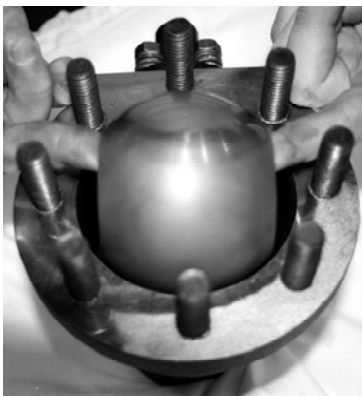
20) Remove the end cap, ball and seat.
